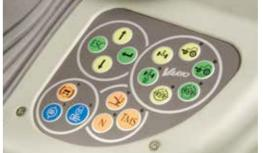
The 3rd and 5th control units can be actuated with the three On the dashboard, you can quickly and easily operate the multiple display, comfort engagement for 4WD, differential lock and front axle suspension as well as the Tractor Management System TMS.
