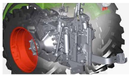
You can control the lateral and tilt adjustment of the swinging power lift, as well as swing and lock, wit
