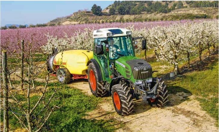
The self-levelling front axle suspension on the Fendt 200 Vario V/F/P specialty tractor quarantees maximum ride comfort, best driving safety and optimum traction. This provides considerable advantages on steep slopes, since all four wheels are in contact with the ground longer.
