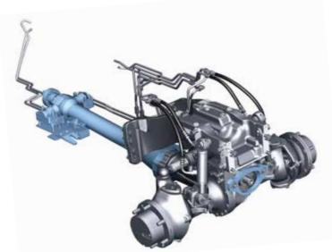
The secret of the exceptional climbing capability lies in the swinging power lift (V/F tractors) and the tractive point that lies in front of the rear axle. With increasing traction requirement, the weight that is transferred to the front axle is also increased. That enables high traction and climbing capability with minimum slip.
