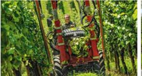
ground reliability and sensibly with FSC. It ensures that working height and lat-ride comfort, even with mounted implements. Driving safety is very high, eral tilt remain constant. Advantage for the driver: calm, relaxed work, because because bouncing is prevented. constant adjustments are not needed.
