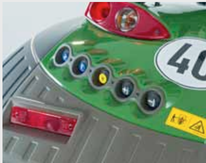
The valves in the Profi version can also be operated externally on the rear mudguard, an advantage when mounting implements.
