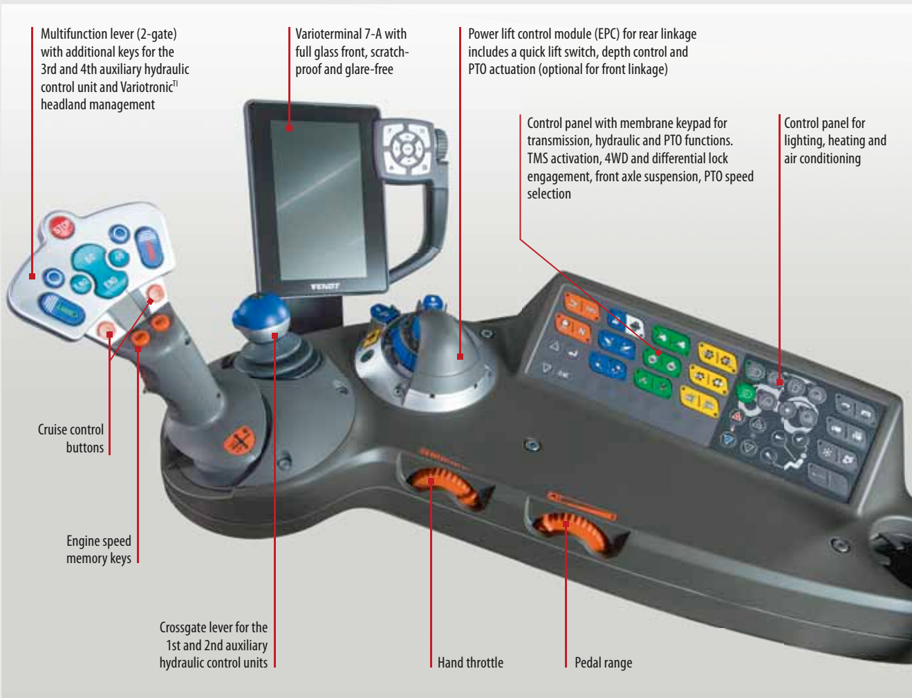
The consistent overall control concept, comprising the Power joystick, power lift control module and membrane keypad, is the ergonomic control centre which allows the operator to keep everything under control.
