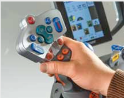
With the two-gate multi-function joystick, you can operate the Fendt 300 Vario like one of the Fendt high-horsepower tractors. The multifunction joystick offers additional control of the 3rd and 4th valves with floating position, headland management (Go, End), second key engine speed memory and cruise control memories C1 and C2.
