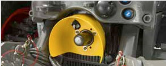
The new integrated front PTO delivers 1000 rpm. The direct drive line from the engine to the implement means high efficiency.
