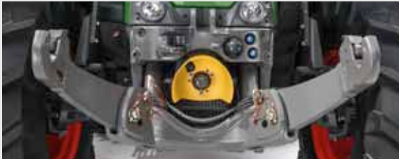
The front linkage is fully integrated in the half-frame and therefore especially stable. The lower links on the front linkage can be folded up diagonally - which provides more free space for front loader work.
