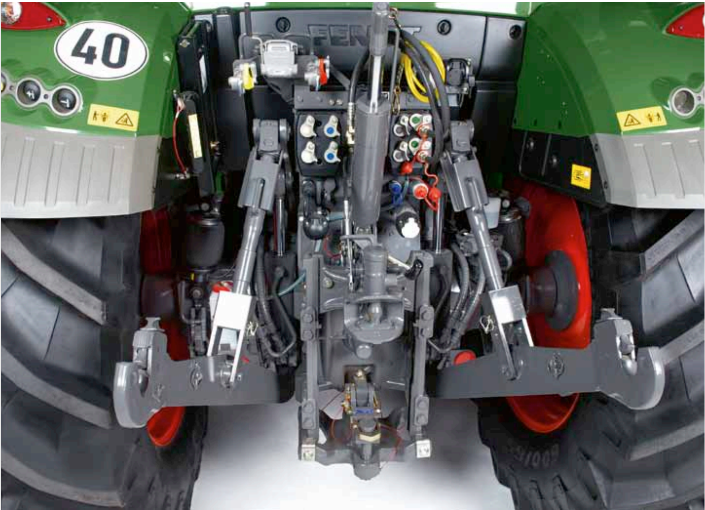
All the interfaces at the rear are arranged functionally and clearly. Signal socket, hydraulic top link, spool valves, unpressurised return, compressed air brake, pressure and control line power beyond, hydraulic trailer brake, 7-pin socket, lower link catch hooks, hitch, rear PTO 540, 540 E and 1000 rpm, bottom hitch, rigid drawbar and much more.
