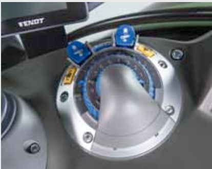
The front lift also has its own valve disc, which means the front linkage does not occupy any of the four spool valves.
