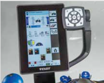
The Varioterminal 7-A unites all the tractor controls, conveniently and functionally, in one terminal. The display, featuring a smartphone design, shows all running functions on a 17.8-cmscreen diagonal with 65,000 colours and a resolution of 480 x 800 pixels. You can navigate easily and quickly through the complete menu using the arrow keys.
