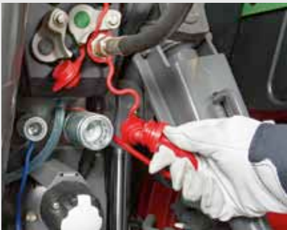
Power beyond pressure and control line for full hydraulic power transmission
