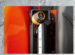
**9x3 Manual Transmission** Manual transmission models feature 9 Forward and 3 Reverse speeds delivering heavy duty performance. Second and Reverse gears are synchronized for efficient forward and reverse operations requiring frequent shifting.
