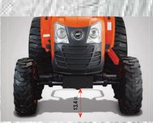
High Ground Clearance The maximum ground clearance of 13.4 in. makes usage on rocky or uneven terrain simpler.
