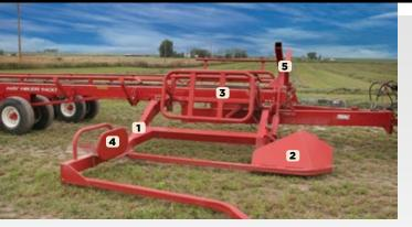
Unique pick on-the-go system - an adjustable, heavy duty bale fork (1) easily lifts today's larger round bales. Dual hydraulic cylinders provide smooth fork operation and full control when picking bales. A bale turner (2) on the inner arm eliminates stress
