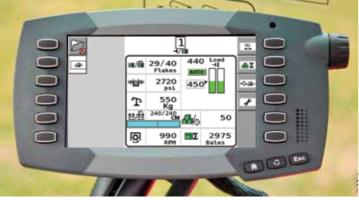
The new Integrated Bale Weighing System (IBWS) is an option that operates through the C1000 baler monitor. This allows the operator to monitor individual bale weight, flake width, bale length and total bale weight, which provides the great benefit of enabling contractors to buy straw or sell forage by the precise tonnage, rather than on a per bale or area basis.
