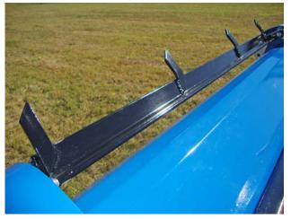
8mm thick angle slats and teeth are the strongest on the market and are designed to operate effectively in both directions and help pull the bale apart. The angle slat gives the teeth a bigger rip area compared to box section
