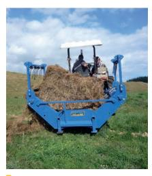
Optional fully adjustable square bale attachment with spring tynes. By being able to adjust both the tyne and angle of the bar the attachment can be adjusted to suit
