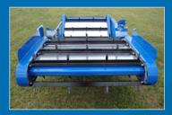
Extended sides on the extension help reduce the product falling off the sides
