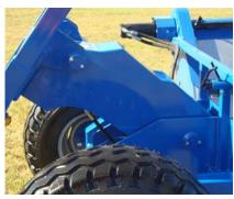
The large lifting arm makes the whole lifting frame very strong when travelling with a bale
