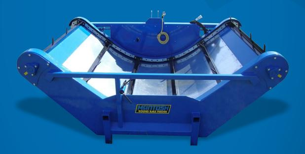
The cradle is intentionally short to help reduce the chance of bales twisting around and taking longer to feed out. The high front and back bars help stop the bale from falling out when travelling and feeding. A short cradle with end bars will feed out better than a long cradle with wasted room and extra weight out the back of the tractor. With no or short end bars bales can twist and fall out.
