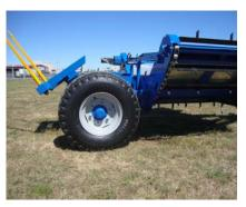
Standard tyres are 11.5x15.3, 50mm taller than the common 10.5x15.3 used on most double bale feeders. The taller tyre tows better over rougher ground than the smaller tyre
